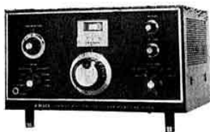
THE JR-500SE Crystal controlled, double conversion receiver. 3.5MHz -29.7 MHz in 7 bands, £68 only. The finest value ever!
