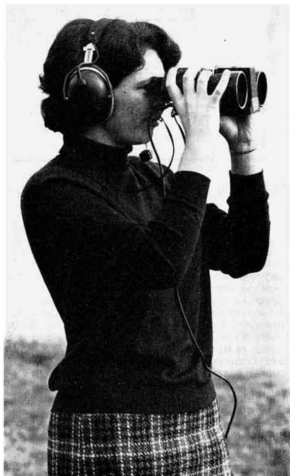
We only need to describe the device she is holding—the SRDE binocular transceiver using a gallium arsenide lamp to work up to \frac{1}{2} mile.
